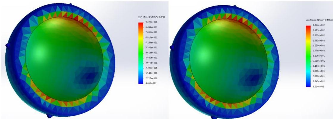
Fig. 2. Stress distribution in polyethylene socket inlays for 100 (left) and 200%BW (right)
