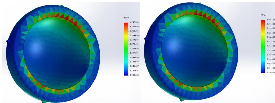
Fig. 5. Deformations in ceramic socket inlay for 100 (left) and 200%BW (right)
