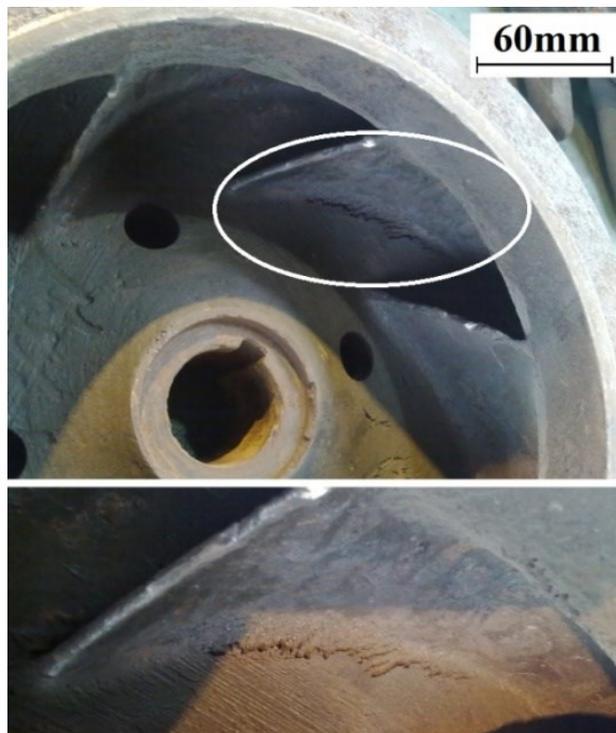
Fig. 3. Cavitation damage of the rotor disk located near the intake edge of the blades.
