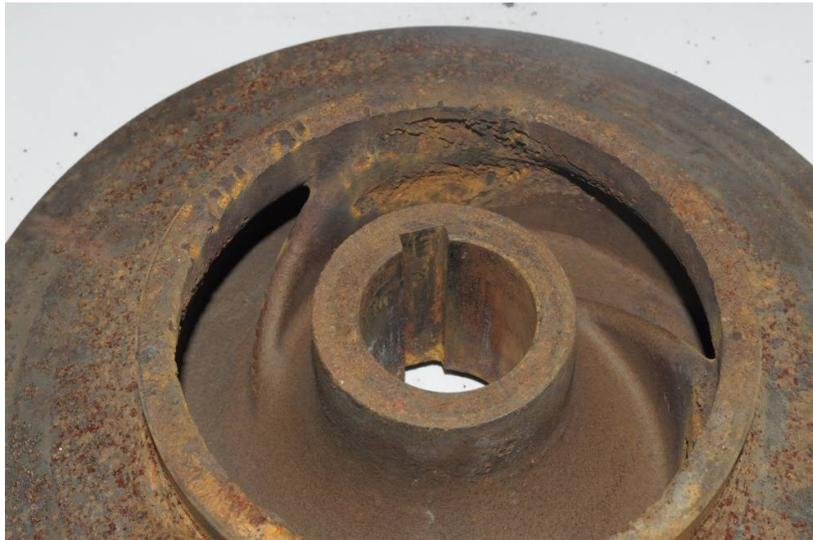
Fig. 2. Centrifugal impeller with a single curvature of the blades.
