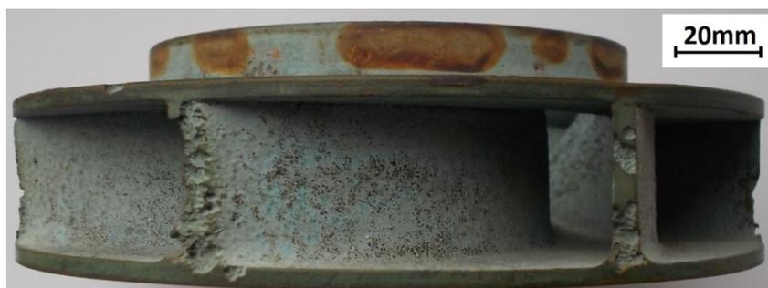
Fig. 4. Centrifugal impeller with a single curvature of the blades.
