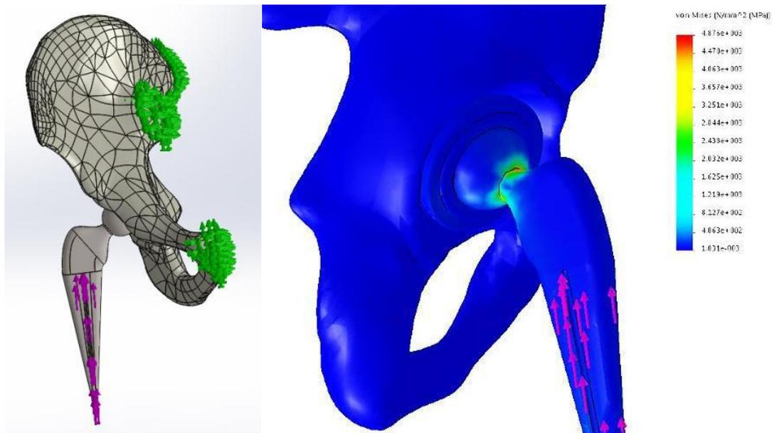
Fig. 7. Fixation points and results of FEM analysis of hip joint endoprosthesis [12]
