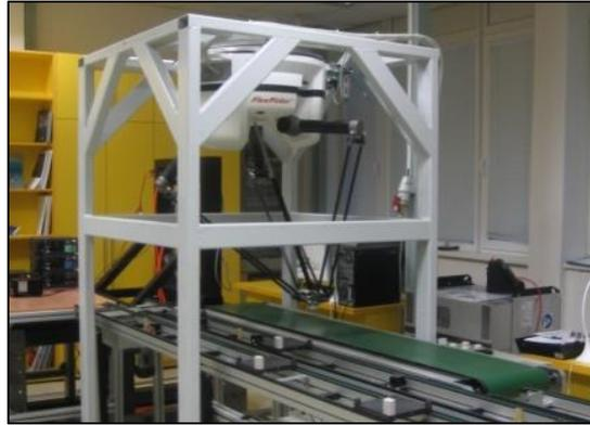
**Fig. 2. Workplace with parallel robot ABB**
