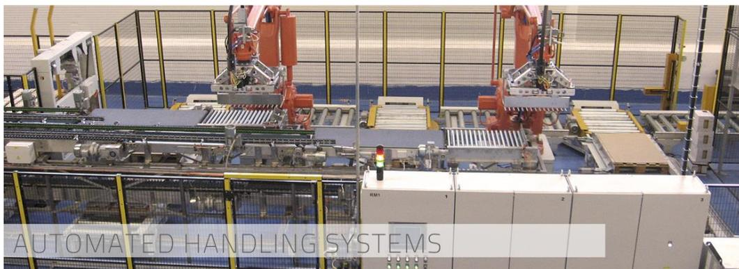
Fig. 2. Palletising robotic workstation
