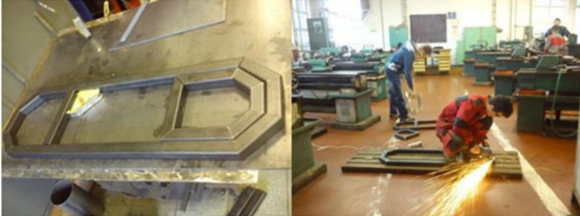
**Fig. 3. Building of off-road wheelchair construction**
