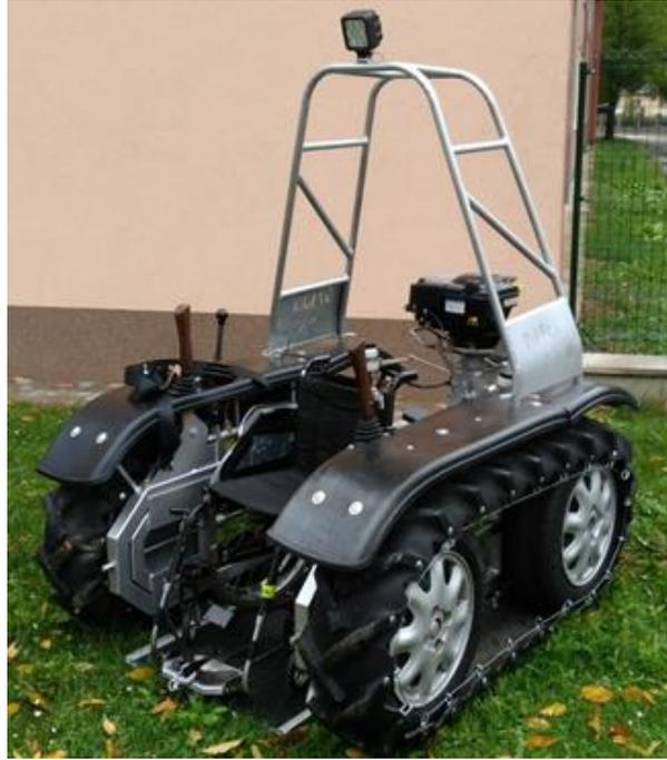
Fig. 4. The prototype of off-road wheelchair
